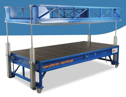
VACUFORM VERTICAL is the fusion of our sophisticated vacuum technology with a vertical movement of 900 mm. This opens new dimensions in terms of functionality and applications – a pressing step forward! Precise pressing results with large, complicated shapes.
