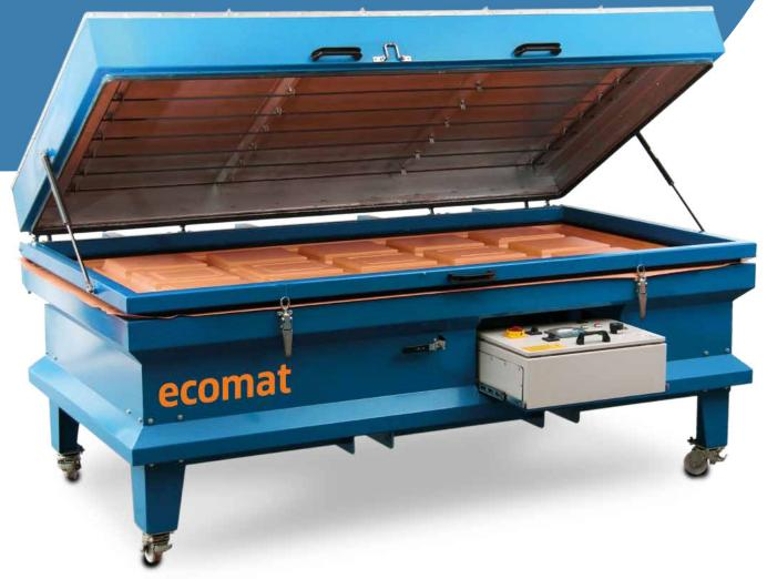
The time and cost-saving 3D-foil laminating technology of the ECOMAT is ideal for laminating kitchen and bathroom furniture, for foil wrapping profiles and special parts such as furniture legs, etc.
